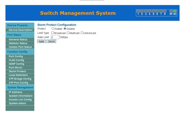
Switch also protects against, for example classic DoS attack (frames with destination address FF:FF:FF:FF:FF)
