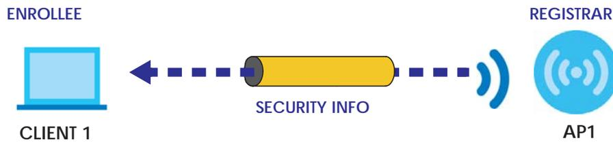
In step 2, you add another wireless client to the network. You know that **Client 1** supports registrar mode, but it is better to use **AP1** for the WPS handshake with the new client since you must connect to the access point anyway in order to use the network. In this case, **AP1** must be the registrar, since it is configured (it already has security information for the network). **AP1** supplies the existing security information to **Client 2**.
