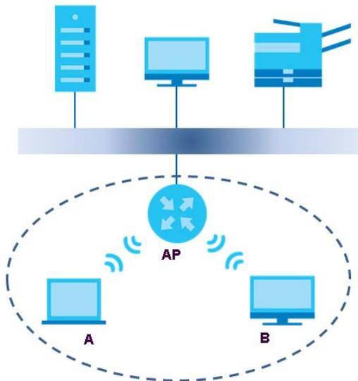
The wireless network is the part in the blue circle. In this wireless network, devices **A** and **B** use the access point (**AP**) to interact with the other devices (such as the printer) or with the Internet. Your LTE4506 is the AP.
