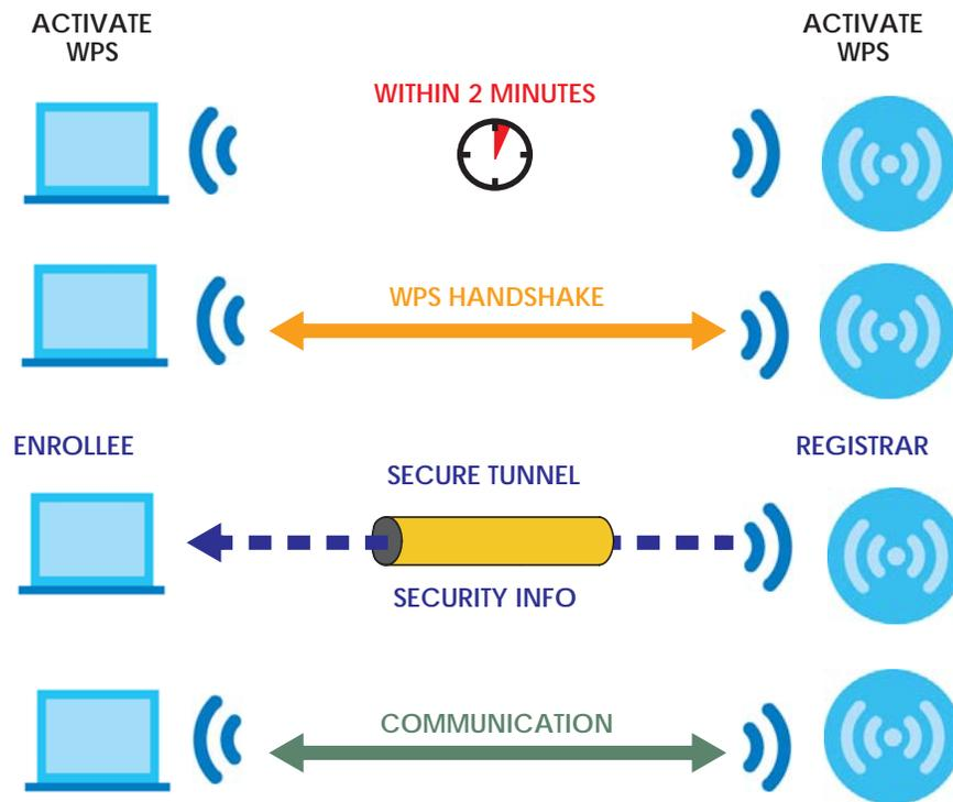
The roles of registrar and enrollee last only as long as the WPS setup process is active (two minutes). The next time you use WPS, a different device can be the registrar if necessary.
