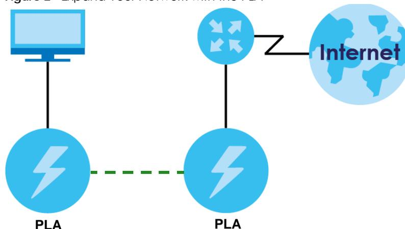
Connect your PLA to an Internet gateway such as a modem and plug it into an ordinary power outlet in your home. Plug a second PLA into another power outlet and connect a computer to the PLA for Internet access. Your network can be further expanded by plugging additional PLAs into other outlets in your home and connecting other computers or network devices (for example, a printer) to them.
