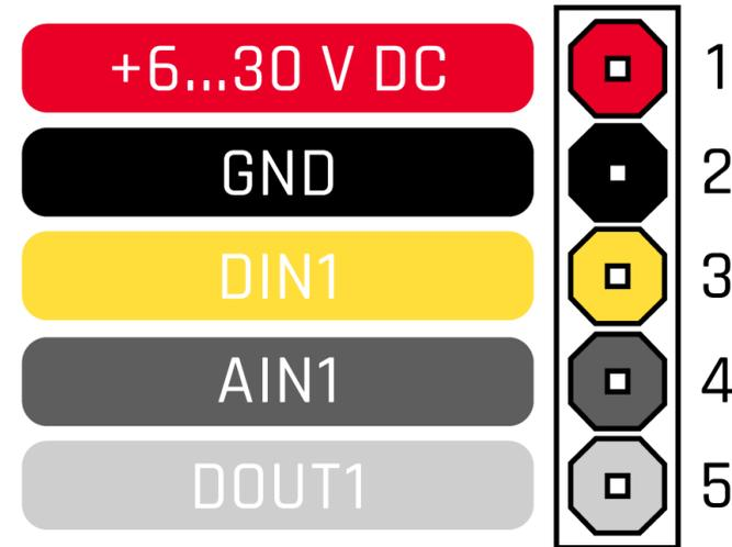
**Figure 2 FMB920 pinout**
