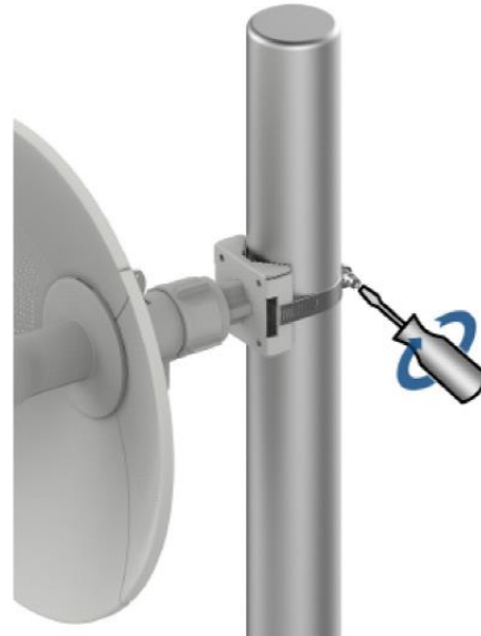
Figure 24 Force 190 mounting bracket (clamp securing)
