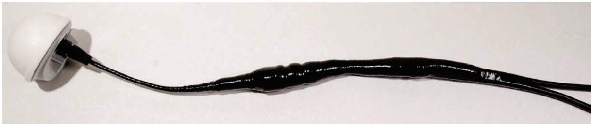
Figure 106 Grounding and weatherproofing example for GPS adapter cable
