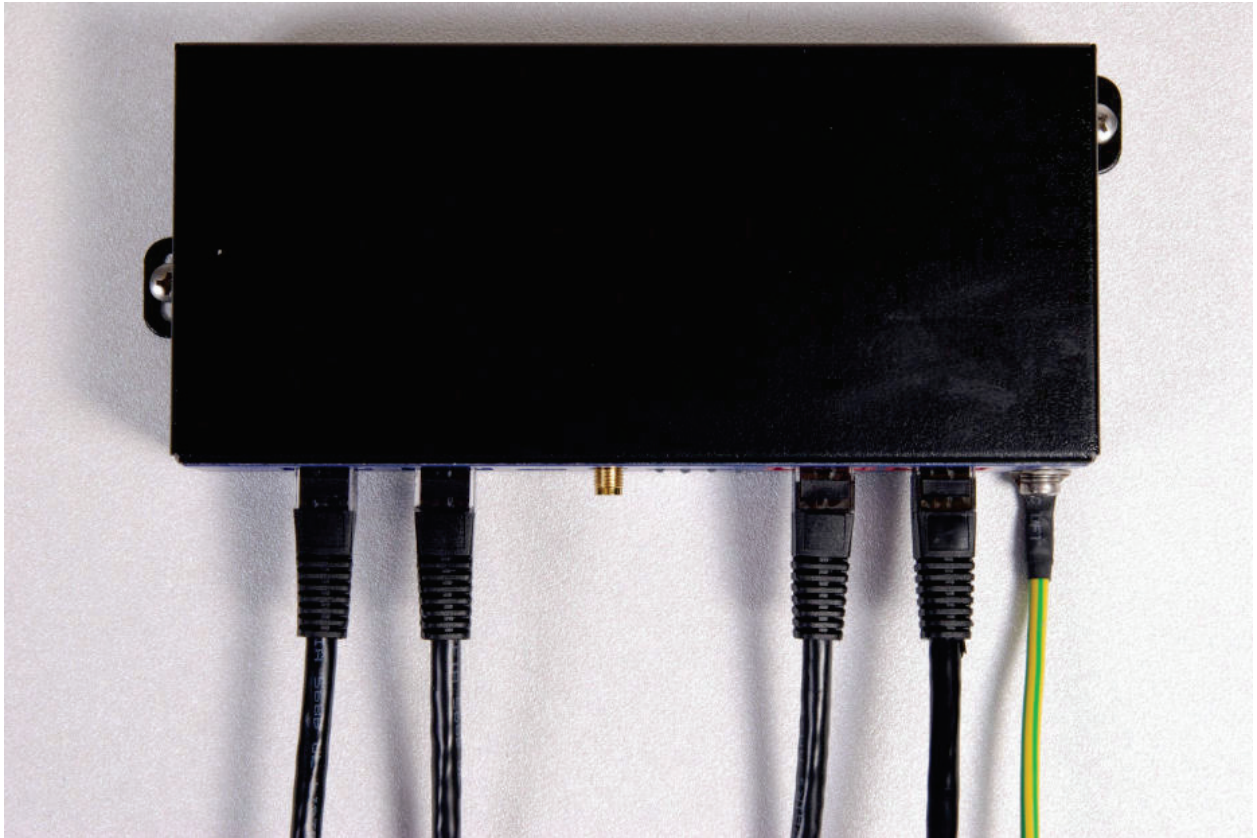
Figure 101 PTP-SYNC mounted on a wall
