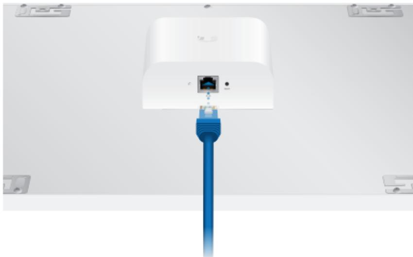
2. Connect the other end of the cable to an 802.3at-compliant switch port that can provide 25W PoE+.
