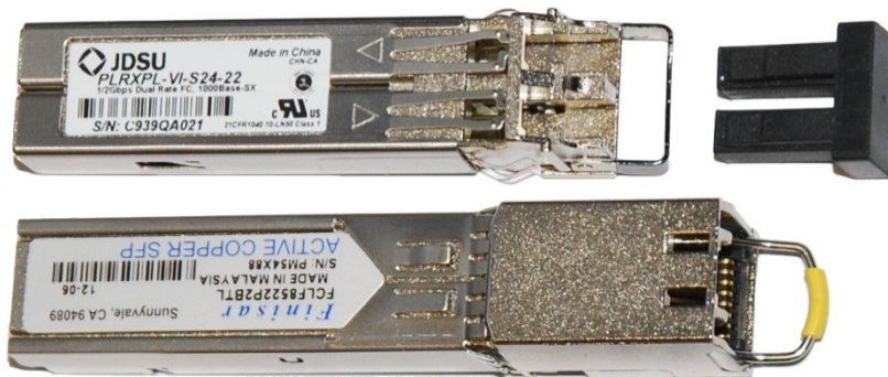
Figure 14 Optical or copper SFP transceiver module
