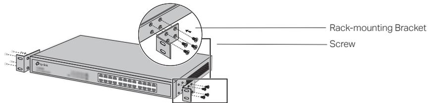
3. After the brackets are attached to the device, use suitable screws (not provided) to secure the brackets to the rack, as illustrated in the following figure.
