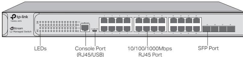
The front panel of The T2600G-52TS is shown as the following figure.
