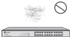
The dust accumulated on the switch can be absorbed by static electricity and result in poor contact of metal contact points. Some measures have been taken for the device to prevent static electricity, but too strong static electricity can cause deadly damage to the electronic elements on the internal circuit board. To avoid the effect of static electricity on the operation of the Switch, please attach much importance to the following items:
