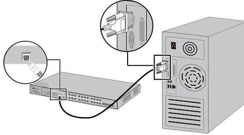
Connect the Console (USB) port of the device with your computer by the USB cable as the following figure shows.
