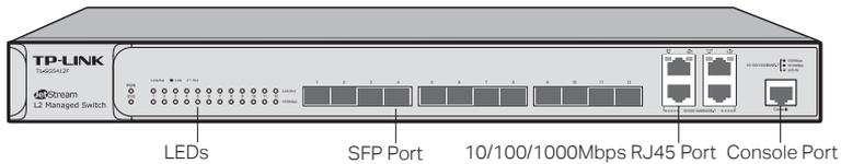
The front panel of T2500G-10TS is shown as the following figure.
