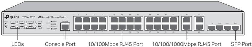
The front panel of T2600G-18TS is shown as the following figure.
