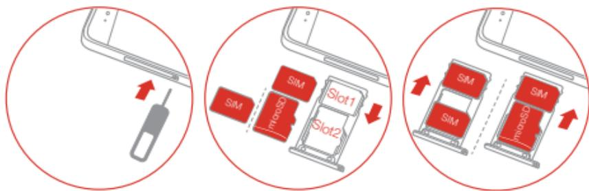
**Step 1.** Insert the eject tool that comes with your smartphone into the hole in the card tray.
