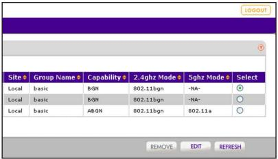
After the access points are added to the Managed AP List, the wireless controller upgrades the firmware of the access points to the latest firmware that is loaded on the wireless controller, and the access points become managed access points. Depending on the number of access points that you add to the Managed AP List, this process might take several minutes.
