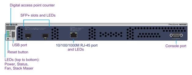
Figure 5. Front panel models WC7600 and WC9500
