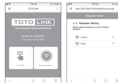
2. Select your router's 2.4GHz and 5GHz primary network and enter the password, then click "connect". It indicates successful connection when the 2.4G/5G green LED remains solid on.
