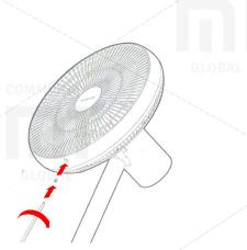
Insert (8) screw into the slot of the main unit and, using a cruciform head screwdriver, tighten it to the limit.
