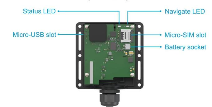
Figure 1 TFT100 device view
