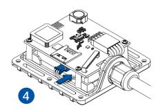
Figure 5 Battery connection
