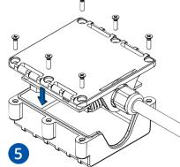
Figure 6 Attaching cover back
