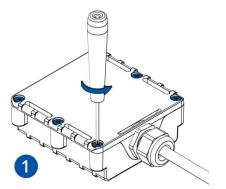
Figure 2 Unscrew screws
