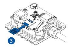
Figure 4 Micro<sub>®</sub>SIM card insert
