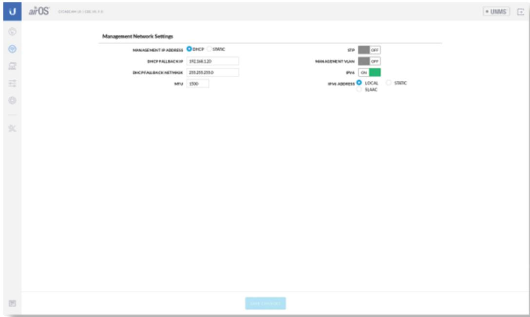
b. Review the Network settings to ensure that each device has a unique IP address. Each can get its IP address via DHCP, or use a static IP address.
