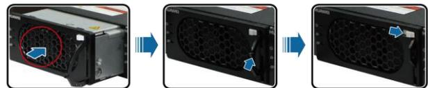
Step 1: Push the locking latch left and pull out the handle.
