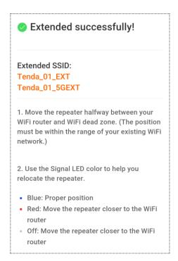
**Step 8** When the Signal LED turns solid blue, A15 is at a proper position.
