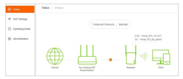
2. Use an Ethenet cable to connect the LAN port of your repeater to a LAN port of your existing WiFi router/modem. The following page appears.
