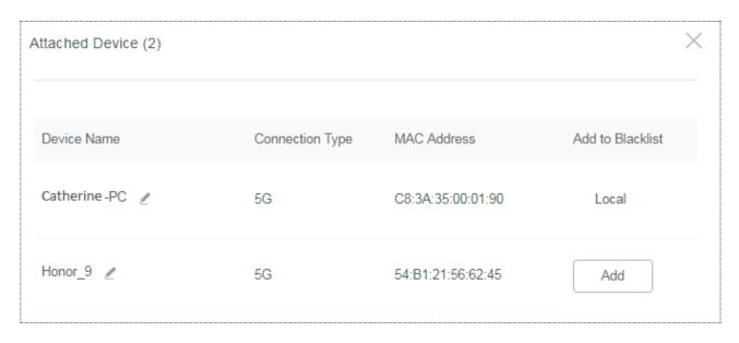
**Add to Blacklist** allows you to block unauthorized or unknown devices. Devices in the blacklist cannot connect to the WiFi network of the repeater.
