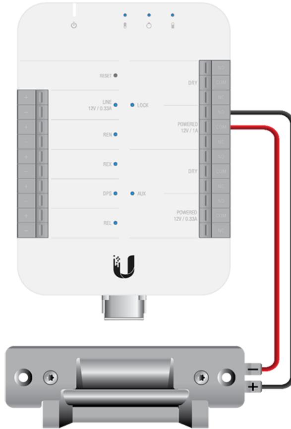
*Fail-secure lock in this diagram refers to electric strike.*
