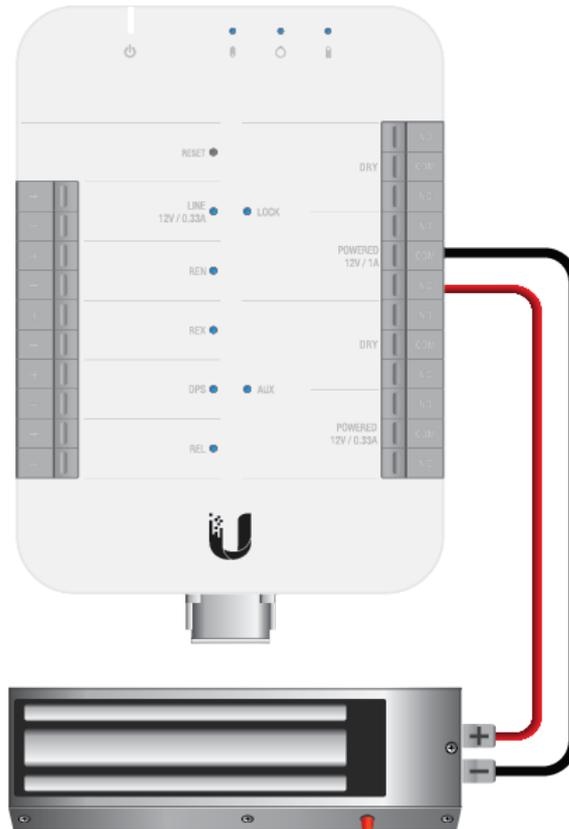
*Fail-safe lock in this diagram refers to magnetic lock or electric bolt.*
