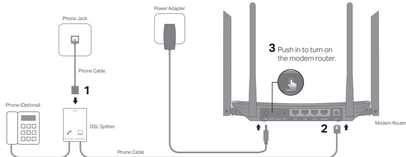
4 Wait for 2 minutes. The Power and DSL LEDs will be on and stable.
