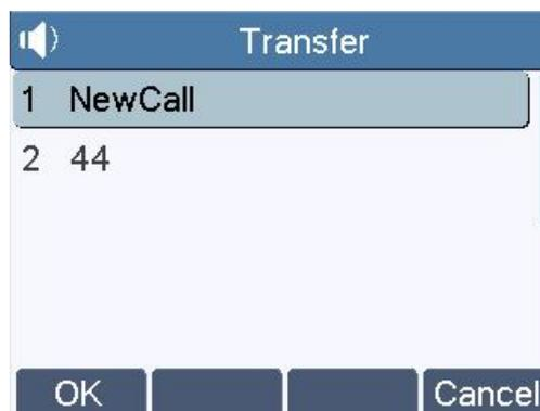
**Picture 26 - Select the line to set up call forwarding**
