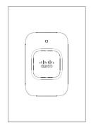
STEP 1 If you are mounting the AP directly to a junction box, go to Step 3. For wall mounting, use the mounting bracket as a template to mark the locations of the mounting holes on the bracket. Figure 1 shows the dimensions of the mounting bracket.
