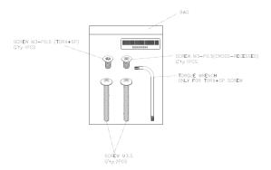
**Note** Make sure all cables are clear and the bracket sits flush against the wall / junction box. The joint created with the screws must have a minimum pullout force of 20 lbs (9 kg).
