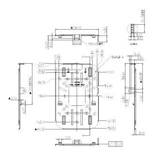
STEP 2 For wall mounting, drill four pilot holes at the mounting hole locations you have marked (at opposite corners of the bracket), and use appropriate anchors as required.
